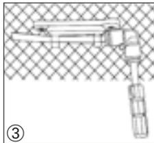
Finally the lead-through can be connected to the incoming and outgoing tubes. The spray heads and the tube can be installed in the terrarium with the help of the suction caps (Picture 1/glass cover) or mounting elements (Picture 2 and 3, wood or gauze).
